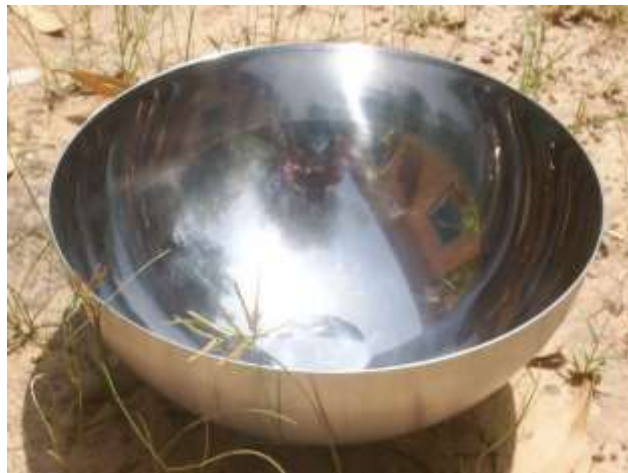
Figure 4: 28 cm diameter IKEA's BLANDA BLANK salad mixing bowl used as solar concentrators.
