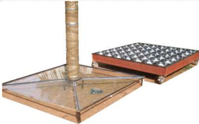
Figure 2: Picture of the 2 parts disassembled solar chimney with the 49 concentrators clearly aligned.
