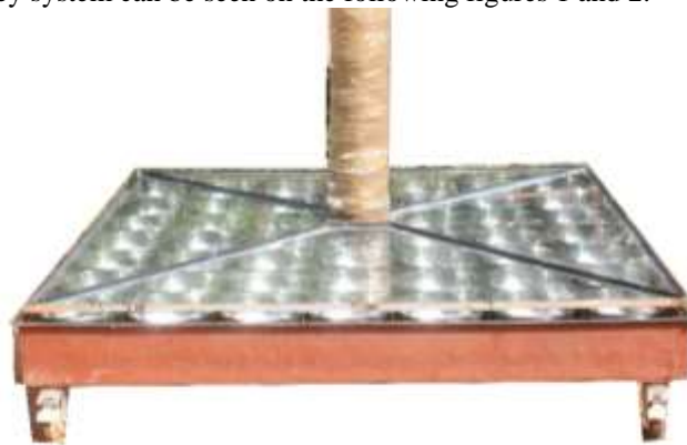
Figure 1: picture of the solar chimney prototype
